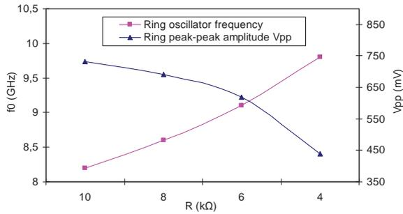
Fig. 5. Dependence of the ring oscillator frequency and the peak-to-peak amplitude  $V_{pp}$  on the feedback resistor value.
